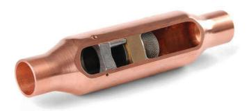
The unit shall use magnetic valves. This valve uses a magnet to hold the valve closed. As the valve opens, the distance between the magnets becomes larger, so the attractive force trying to close the valve diminishes.
